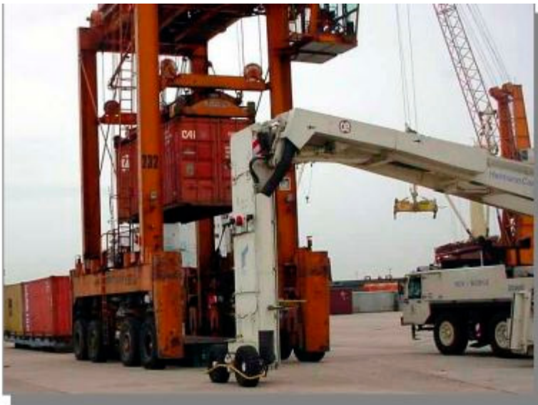
Figure 3. Cargo Container being examined by portable VACIS system
