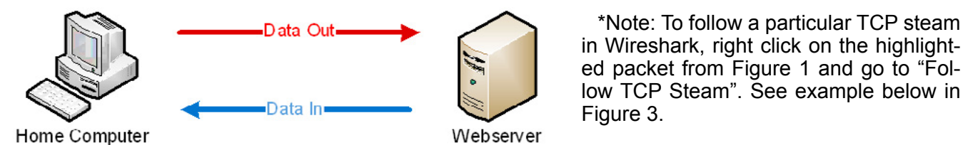
Figure 2. A visual representation of the flow of data in a TCP session
